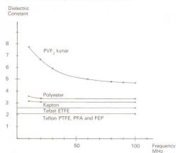
Habia high performance insulations in Teflon, Tefzel and Kapton have a low dielectric constant giving lowest loss, low attenuation and highest possible signal transmission speed.
