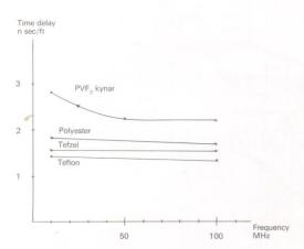
The delay time is significant lower for Teflon and Tefzel insulated wires, than for other common used insulation material.
