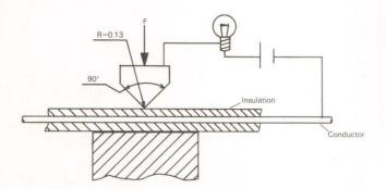
To present the mechanical properties of Tefzel a cut-through test is done, which shows that Tefzel is a very tough isolation.
