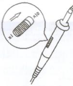
Connect the contact probe with the oscilloscope. Set the attenuation switch to the correct position.
