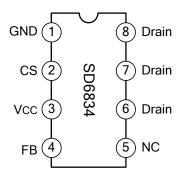
Note: it is □ecommended to connect pin 5 to pin Drain for better heat dissipation.
