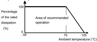
Figure-1 Derating curve
