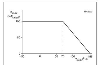
Fig.3 Maximum dissipation ( $P_{max}$ ) in percentage of rated power as a function of the ambient temperature ( $T_{amb}$ ).
