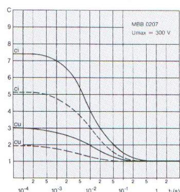
Example: Pulse load rating for long term operation ( $\theta_a = 125^\circ\text{C}$ )
