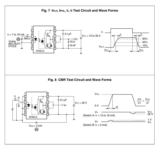
**Remark** CMR Test : Connect pin 1 and pin 4 to the LED common.
