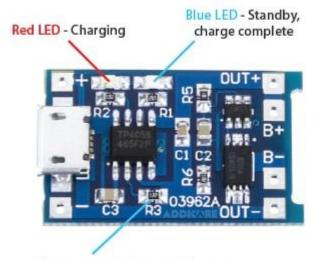
Rprog - constant current charge configuration resistor
