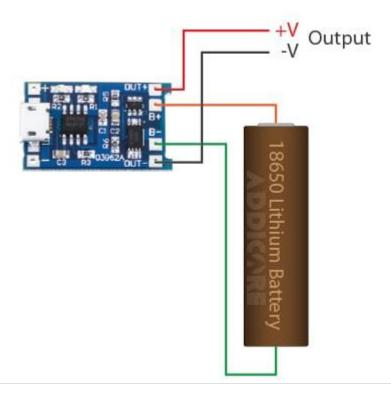
This module is made for charging rechargeable lithium batteries using the constant-current/constant-voltage (CC/CV) charging method. In addition to safely charging a lithium battery the module also provides necessary protection required by lithium batteries. See below concerning the protection features this module provides.
