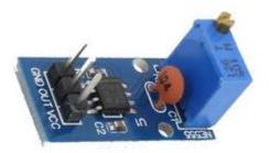
NE555 is a Pulse Frequency Duty Cycle Adjustable Module Square Wave Signal Generator. The output frequency range is selectable. Duty cycle and frequency is not separately adjustable, adjusting the duty cycle will change the frequency. Single channel signal output, the output square wave duty ratio is about fifty percent.
