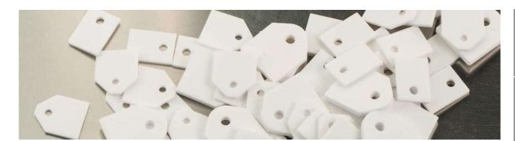
Aluminium oxide slices are used for insulated assembly of semiconductors for high voltage ranges. Despite the high dielectric strength, good heat transfer, from the semiconductor to the heat sink is available.
