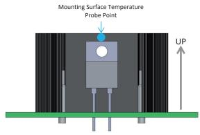
These data relate to a normal application condition with fins obstructed by a PCB and non-ducted airflow, and may be used for practical thermal design.
