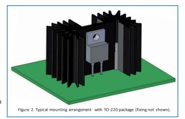
The package should be fitted to the heatsink using a suitable thermal interface material, for example a thermal pad or paste such as Dow Corning DC340. It should be secured with an M3 mounting screw tightened to give void-free thermal contact and to a maximum torque of 0.9Nm.
