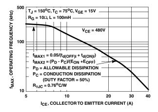
T<sub>C</sub> = 150°C, V<sub>GE</sub> = 15V, R<sub>G</sub> = 10Ω
