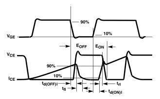
FIGURE 19. SWITCHING TEST WAVEFORMS
