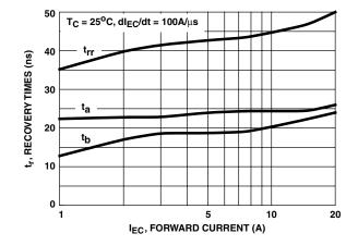
FIGURE 17. RECOVERY TIMES vs FORWARD CURRENT
