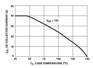
FIGURE 3. DC COLLECTOR CURRENT vs CASE TEMPERATURE
