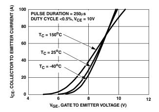
FIGURE 1. TRANSFER CHARACTERISTICS
