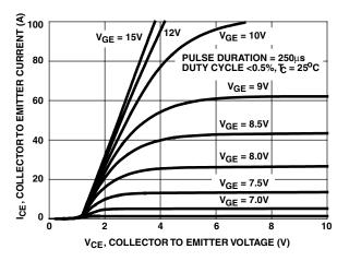
FIGURE 2. SATURATION CHARACTERISTICS
