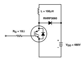
FIGURE 18. INDUCTIVE SWITCHING TEST CIRCUIT
