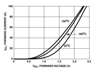
FIGURE 16. DIODE FORWARD CURRENT vs FORWARD VOLTAGE DROP
