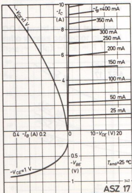
**Transfer, output and input characteristics**
