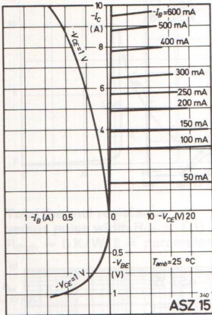
**Transfer, output and input characteristics**
