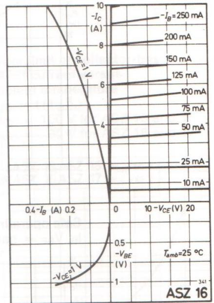
**Transfer, output and input characteristics**
