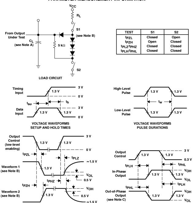
NOTES: A.  $C_L$  includes probe and jig capacitance.
