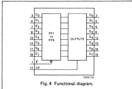
Fig. 4 Functional diagram.
