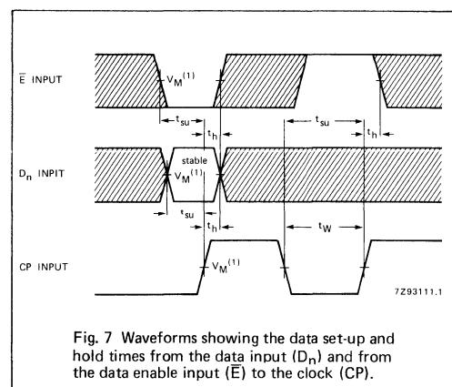
Fig. 7 Waveforms showing the data set-up and hold times from the data input ( $D_n$ ) and from the data enable input ( $\bar{E}$ ) to the clock (CP).
