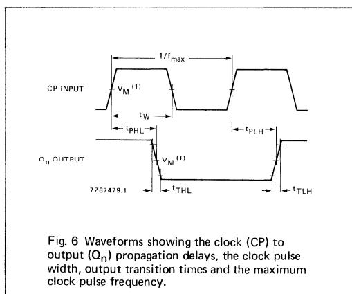
Fig. 6 Waveforms showing the clock (CP) to output ( $Q_n$ ) propagation delays, the clock pulse width, output transition times and the maximum clock pulse frequency.
