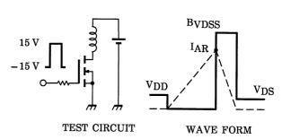
$$\begin{aligned} R_G &= 25~\Omega \\ V_{DD} &= 90~V,~L = 60~mH \end{aligned} \qquad E_{AS} &= \frac{1}{2} \cdot L \cdot I^2 \cdot \left( \frac{B_{VDSS}}{B_{VDSS} - V_{DD}} \right) \end{aligned}$$
