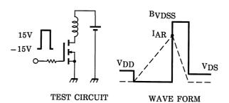
$$\begin{aligned} &RG = 25~\Omega \\ &V_{DD} = 90~V,~L = 27~mH \end{aligned} \qquad E_{AS} = \frac{1}{2} \cdot L \cdot I^2 \cdot \left(\frac{B_{VDSS}}{B_{VDSS} - V_{DD}}\right)$$
